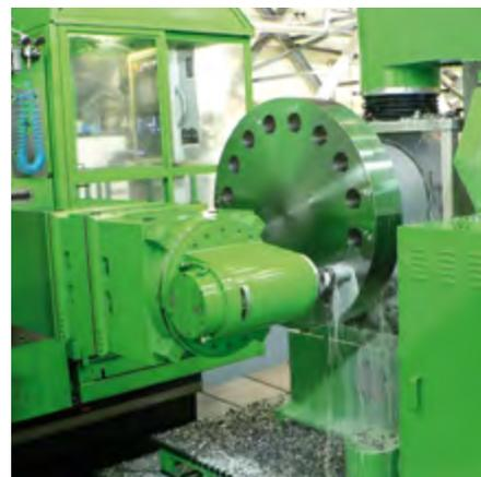
Machining of coupling holes
