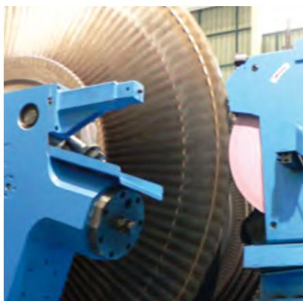
Grinding of turbine's blades
