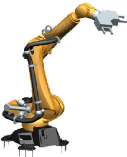
RTC allows exchange of tools to machine spindle or to spindle of various milling heads indexed under any angle. This saves the additional changing time required for positioning of the head to the loading position. Actual number of tools is practically unlimited thanks to using of storage tool area for hundreds of different tools. RTC also allows other additional functions such as fast automatic tool break monitoring system or others.
