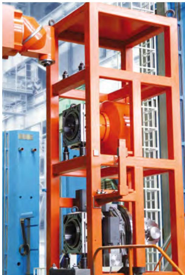
Head pick up system for Automatic Attachment Changer (AAC)
