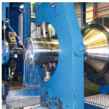
Machining of windmill shaft
